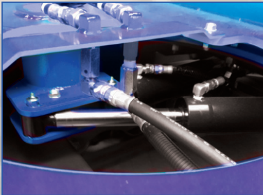
CONTROL OF THE TURN- TABLE WITH 2 HYDRAULIC CYLINDERS
