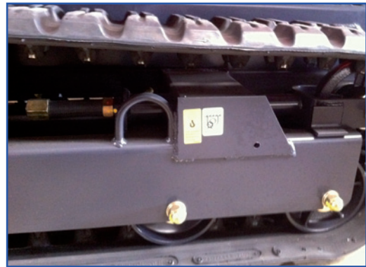
SIMPLE CHAIN TENSIONING SYSTEM
