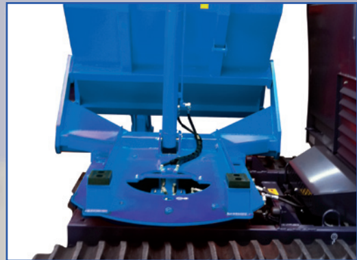
TURNFUNCTION: TURNABLE WORKS WITH 2 HYDRAULIC CYLINDERS
